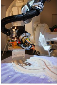
Robotic Tooling of a plaster running mould with realtime projectionmapped feedback.
